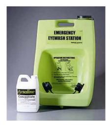
An emergency eyewash station is defined as one that provides a continuous flushing fluid to both eyes at a minimum of 1.5 L per minute for 15 minutes. It can be plumbed in or portable. Portable bottles (squeeze bottles) do not meet this standard. Squeeze bottles, however, are also to be made available for all activities where there is risk of materials entering the eye.
